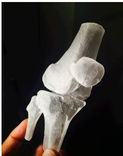
Figure 1. A knee joint printed with clear 3D filaments t-glass on a Makerbot Replicator 2X at the University of Ottawa. The knee joint model was extracted from computed tomography (CT) data.
